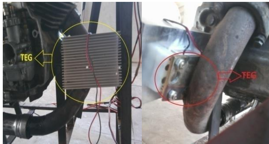
Fig-4: Front and rear view of the TEG in the system
